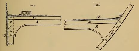
'Tween-deck Stringer.—Have all beams in and riveted before commencing to put in 'tween-deck stringers.
